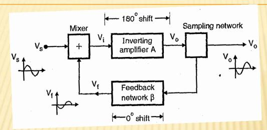
The block diagram of an amplifier with a Negative Feedback Fig.
